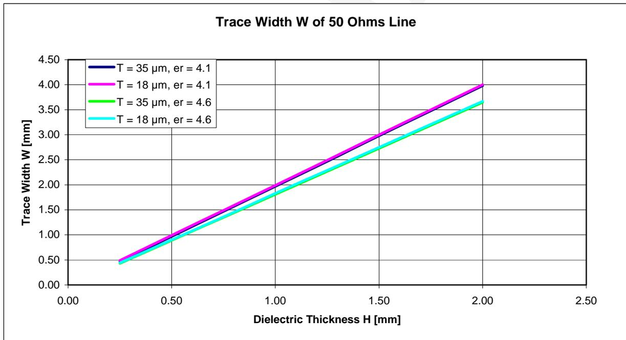
Figure 3-4: Dependency of Trace width of a 50 Ohms line on dielectric constant  $\epsilon_r$ , and copper plating thickness T
